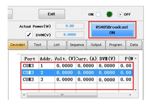
Monitoring software of this series power source add global control function. With RS485 communication, it is available to connect 30 units of different models and there are two ways to set output parameters:
