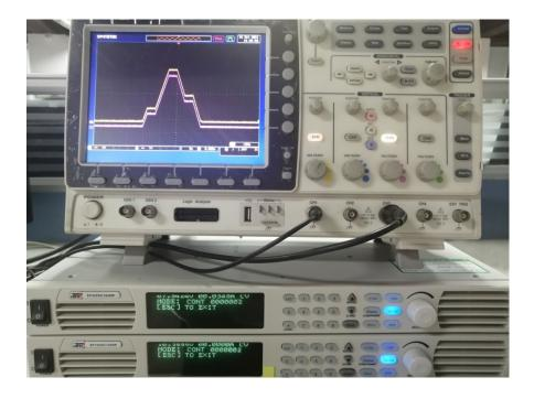
Via serial pot test tool, send output parameter to each power source. Using global command CALL to realize control multiple power source output.
