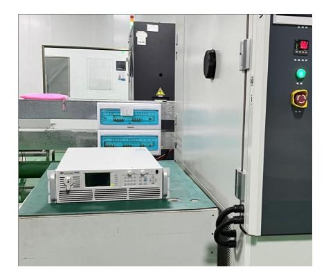
SP-3U/6U series power supply has high precision, high stability, CC mode and analogue output which could apply in long time quality and performance test to new energy automobile component.
