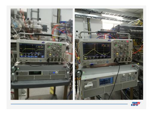
Slew rate of current is adjustable which is easier for user to use.
